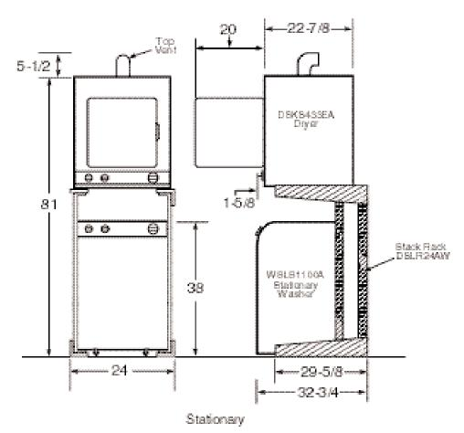
Washer Note: Washer wall outlet must be located within 36" of service cord entry. Wall outlet must not be located behind dryer.
