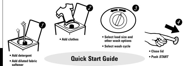
NOTE: When making a selection with any knob, simply point the knob anywhere within the shaded range for that setting.
