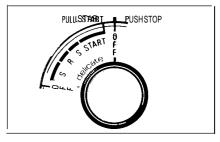
To get the full benefit of the Delicate Cycle, always set it at the beginning of the cycle. During wash, the Delicate Cycle alternates between agitation and pauses to protect delicate clothes.
