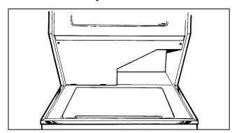
Lift access panel up until tabs at sides of panel slip out of slots at sides of dryer.
