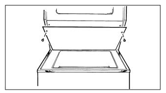
Remove two Phillips-head screws at top of panel.
