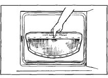
Remove the lint filter by pulling straight out. Wipe all accumulated lint from screen. Occasionally wash filter using soap and warm water. Rub lightly, rinse and dry thoroughly. This will help remove all fabric softener buildup.
