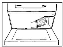
Lift access panel up until tabs at bottom of panel slip out of slots at rear of washer.
