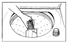
• Agitator. Remove the agitator at regular intervals-about 4 to 6 months—and remove any lint that may have accumulated. After removing the front access panel, as shown at right, unscrew the agitator cap, grasp the agitator with both hands, and pull it up and out of the washbasket.
