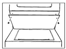
Remove two Phillips-head screws at top of panel.
