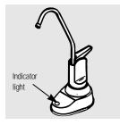
**Electronic Indicator Light**—The electronic indicator light on the base of the faucet is a six month timer that shows you when to replace the filter cartridges. When the battery pack is first installed, the indicator light will light briefly to show that the electronics are operating. If this does not happen, the batteries could be installed backwards or the leadwires are not connected.
