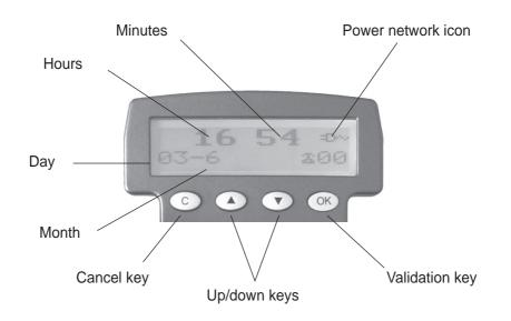
OK button is used to confirm action or a choice on the screen.
