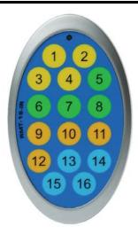
Buttons 1 through 8 on the RMT-16 IR remote control correspond to display outputs A through H. Buttons 9 through 16 correspond to source inputs 1 through 8. Please use the steps and chart below for instructions on how to route video sources to displays.
