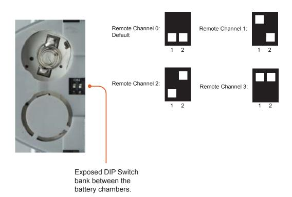
It is important that the IR channel on the Remote Control unit, matches the IR channel set on the 16x16 3GSDI Matrix. For example, if both DIP switches on the IR Remote Control unit are set to IR channel 0 (both DIP switches down), then the 16x16 3GSDI Matrix must also be set to IR channel 0. See page 22 on how to change the IR channel on the 16x16 3GSDI Matrix.
