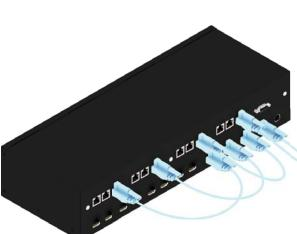
When all jumpers are connected, extension for each HDMI output is possible. If a local display is going to be used, simply do not use that HDMI output port's jumper and extension connection.
