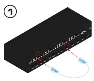
This example shows the jumper connection between HDMI output port 1 and HDMI extension input port 1 .
