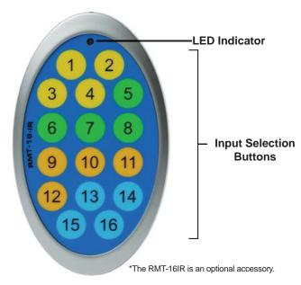
The RMT-16IR remote control will allow the user to select which source will be routed to which output. Each of the 4 outputs are assigned a group of 4 buttons that will correspond to the 4 source inputs. Each button on the RMT-16IR remote control will toggle between the "A" and "B" sources for each input. Please use the information below when selecting the desired source for each display. The LED will blink each time a button press is detected
