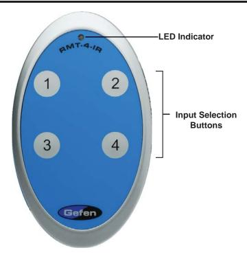
Pressing on each numbered selection buttons will switch the receiver to the corresponding HDMI Input source. Each input can have up to 2 sources connected (A and B). Each press of a input button will toggle between the A and B source. The LED will blink each time a button press is detected.
