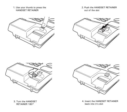
Figure 3 Handset Retainer for Wall Mounting
