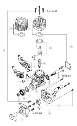
\*Type of screw C···Cap Screw M···Oval Fillister-Head Screw F···Flat Head Screw N···Round Head Screw S···Set Screw
