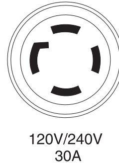
Figure 8 - 120/240 VAC, 30 Amp Receptacle
