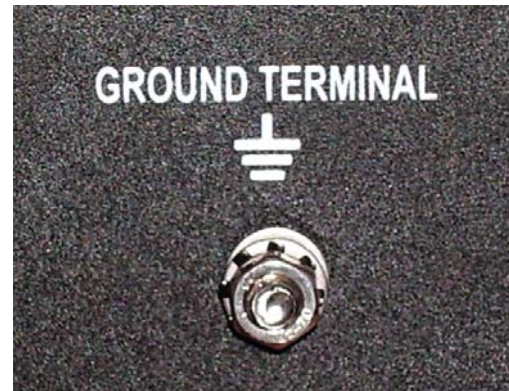
Figure 7 - Grounding the Generator
