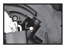
The generator was configured for natural gas operation at the factory. Switching over to LP vapor is a simple procedure.
