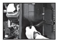
Finally, insert the plastic plug that came with the generator into the hole on the bottom of the air cleaner base.
