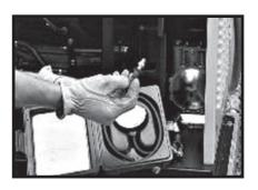
Check the gas pressure at the secondary regulator to make sure there's enough pressure for proper generator operation.
