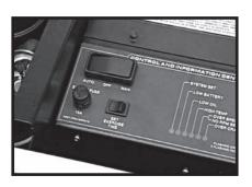
With the mode switch in AUTO, press the EXERCISER switch. Hold it down for at least 10 seconds and release. The generator should start within a few seconds. The unit will run for about 12 minutes before shutting itself down automatically.
