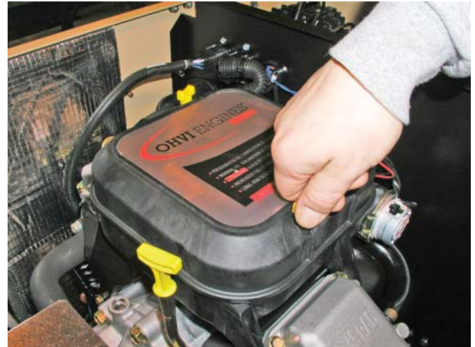
Figure 2.2 – Restrict Air Flow During Initial Start Up
