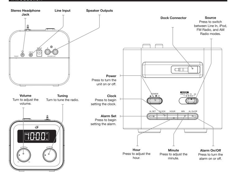
Plug the included AC/DC power adapter into the DC POWER INPUT on the dock and an AC power outlet to power the dock.
