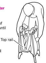
FOR SMOOTH SETUP and takedown, it's important to remember one thing: the center of the floor must be at least halfway up when locking OR unlocking rails (see picture below). Therefore:
