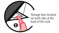
3. Fasten ends of tether and **lower anchors** onto their respective storage bars as shown **2**.
