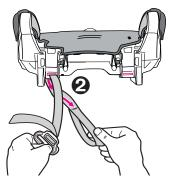
2. Pass the clip and the strap through the loop end ③ as shown and pull strap up.
