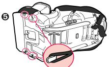
5. Pull elastic loop on the seat pad through the vehicle belt guide on side of seat and attach to hook as shown **3**. Repeat on other side.
