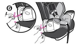
6. Squeeze height adjust button ② and push head support into slots ③ on the back support as shown. Head support will click into the back support.
