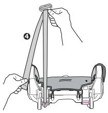
4. Slide the vehicle shoulder belt onto the clip as shown  $\odot$  and pull free end of strap down  $\odot$  to tighten clip against the child's shoulder.
