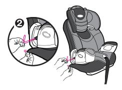
3. Pull the seat pad out of the way to reveal red buttons as shown in **3**. Slide the buttons to release the back support from the base and lower it into a flat position.
