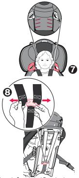
7. Pull strap ends through slots at front of seat ② and reinsert them in the desired slots ③. Check that the straps are not twisted.
