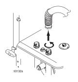
Loosen bolt (A) located between air and material hose outlets. Unscrew bolt to lower plate, leaving about 4-5 threads on bolt.
