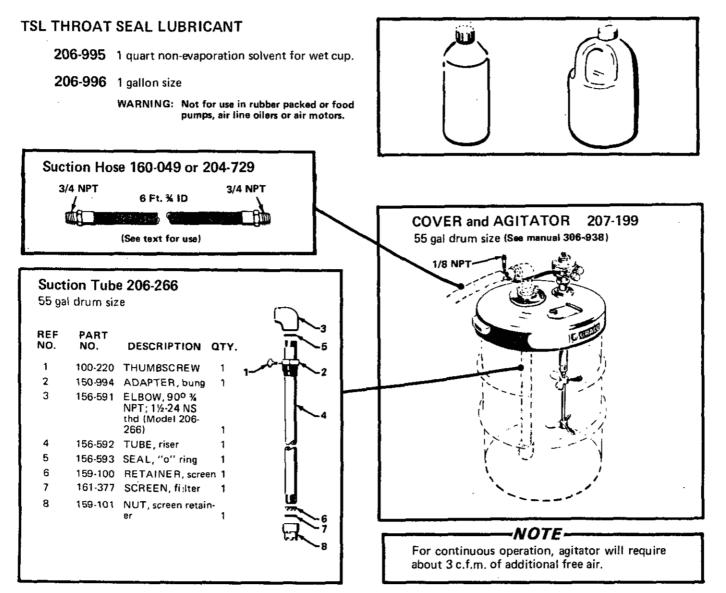
For agitation of paint and suction directly from original 55-gallon shipping container. 6-ft. suction hose 160-049 is for petroleum base solvent flushing and water base materials: 204-729 is for hydracarbon solvent flushing materials.
