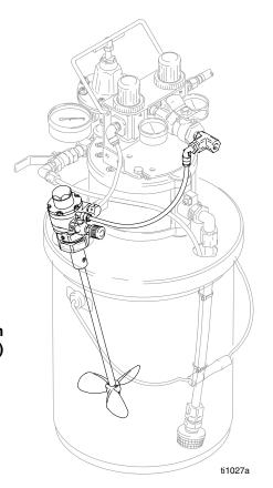
Agitator Kit shown installed on TRITON 308 spray package (not included)
