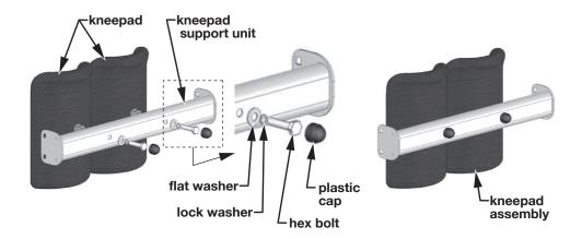
2. Insert the kneepads into the kneepad support unit. Install the two hex bolts through lock washers, flat washers, and kneepad support unit into nuts as shown above. Tighten securely with the provided wrench. Install the two plastic caps on the hex bolts. The finished assembly is shown at right above.
