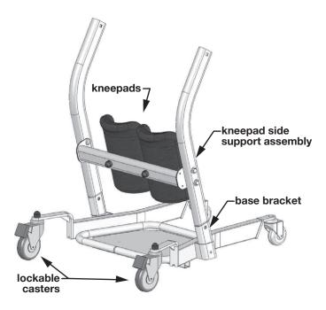
5. Insert the kneepad side support assembly into the base brackets as shown above. The kneepads and arm curvature should be facing away from the lockable casters.
