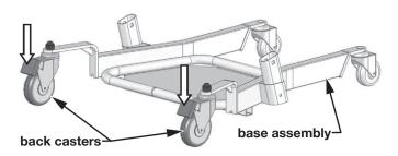
1. Place the base assembly on the floor and lock the back casters for ease of assembly, as shown above.
