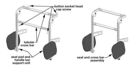
4. Insert the two tubular cross bars into the holes on the seat pad and handle bar support units as shown above. Align the small holes on the cross bar undersides with the holes in the support units. Install the four button socket head cap screws through the support units into the cross bars. Use the hex key to tighten. The finished assembly is shown at right above.
