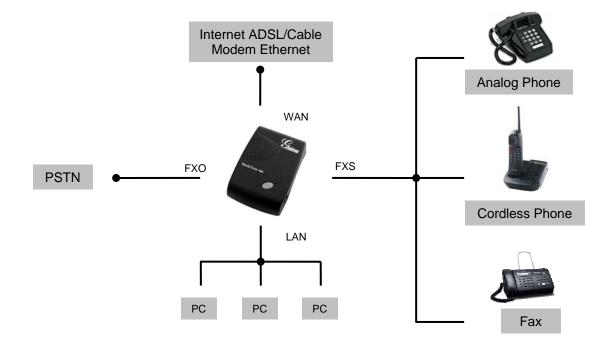
HandyTone-488 has one FXS port and one FXO port. The RJ11 jack next to the LAN port is a FXS port. The RJ11 jack on the side of the HandyTone-488 is a FXO port. Both the FXS port and the FXO port can have a separate SIP account. This is a key feature of HandyTone-488. Telephone calls can be originated or terminated from/to the PSTN network via FXO port.
