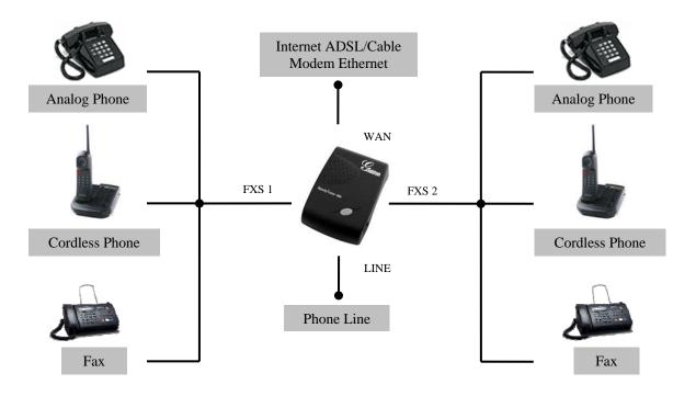
HandyTone-386 has two FXS ports. The RJ11 jack next to the WAN is called FXS port 2 and the RJ11 jack on the corner is called FXS port 1. The RJ11 jack on the side on of the HandyTone-386 is a LINE port. Each FXS port can have a separate SIP account. This is a key feature of HandyTone-386. Both ports can make calls concurrently.
