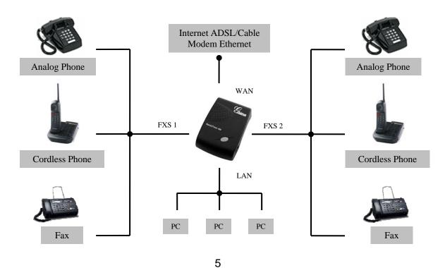
HandyTone-496 has two FXS ports. The PHONE1 port next to the LAN is FXS port 1 and the PHONE2 on the side of the HandyTone-496 is FXS port 2. Each FXS port can have a separate SIP account. This is a key feature of HandyTone-496. Both ports can make calls concurrently.
