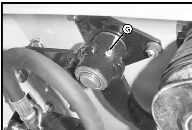
6. Grease traction drive belt tension arm pivot (G).
