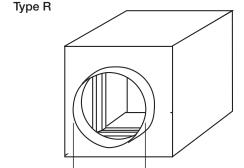
Type R transition is centered on damper frame. Dimensions are with 2 in. (50mm) offset.
