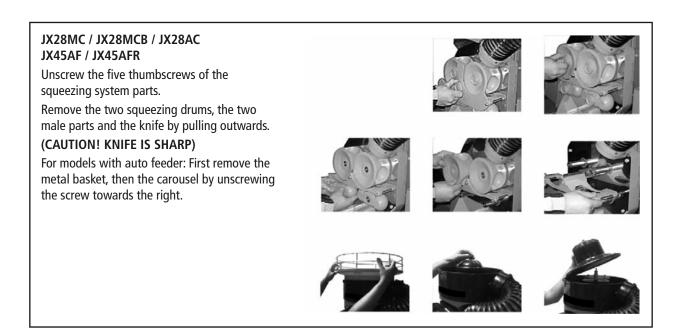
Clean all parts and the body of the machine with water and detergent. Do Not Use Abrasive Cleaning Products, they can damage the parts. Dry the parts and the interior of the machine.
