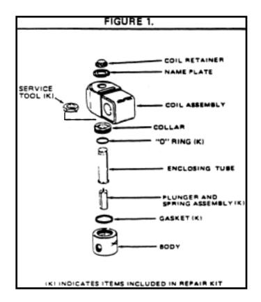
As with all valves, it may become necessary to clean them periodically to keep them in peak operating condition. Any cleaning methods or fluids used should be compatible with valve materials.
