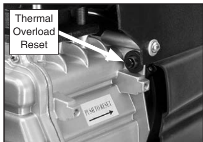
Figure 8. Thermal overload reset.
