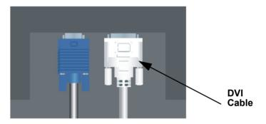
5. Connect the DVI connector at the other end of the signal cable to the DVI port located on the back of the graphics adapter. See picture below
