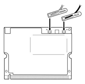
**Note:** Plug the gray antenna cable with the tab marked "MAIN" into jack M, and the black antenna cable with the tab marked "AUX" into jack A.
