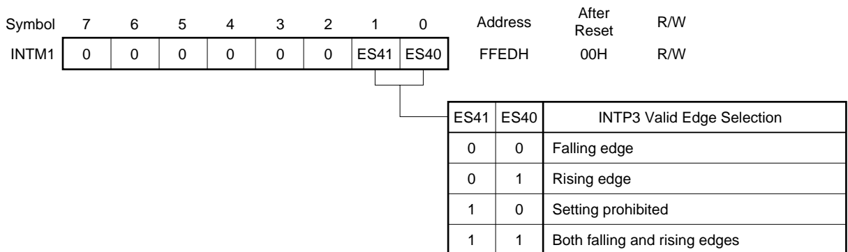
Figure 12-6. External Interrupt Mode Register 1 Format
