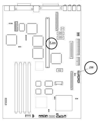
2. To disable the external SCSI connector, move the jumper on J35 to the front two pins, and move the jumper on J36 to the rear two pins.
