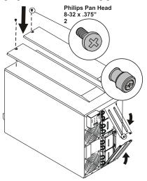
**2** Bring the unit to tower position, and remove the display bezel by sliding to the left and out. Rotate the display bezel and reinstall. Install the first battery module at the bottom.
