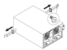
**3** Reinstall the remaining three battery modules.
