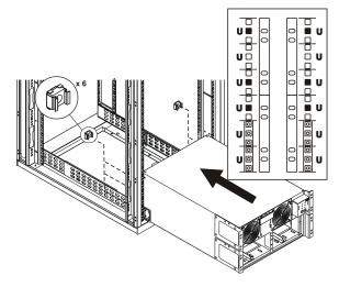
3 Secure the uninterruptible power supply in the rack.
