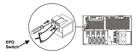
Both Class 2 and SELV circuits must be isolated from all primary circuitry. Do not connect any circuit to the EPO terminal block unless it can be confirmed that the circuit is Class 2 or SELV.
