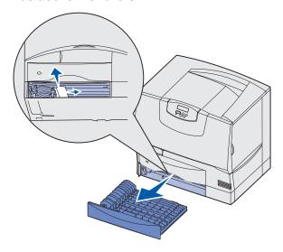
2 Reinstall the duplex mechanism in the printer.
