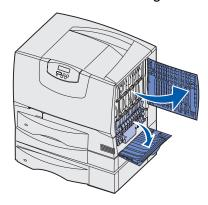
**3** Pull down the latches. They slide toward the center to release the fuser.
