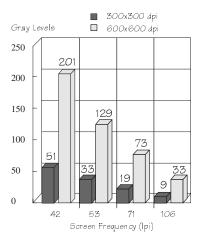
The number of gray levels that your printer can produce depends on the screen frequency and the print resolution. The default value for screen frequency using 600 dpi is 71 lpi. This typically allows 73 different levels of gray. The default value for screen frequency using 300 dpi is 53 lpi. This typically allows 33 different levels of gray.
