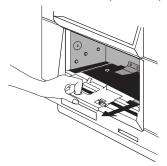
6 Remove the two screws on the duplexing unit slot-cover.
