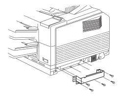
5 Remove the metal cover revealing the tray assembly.
