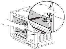
4 Insert a finger or a screwdriver in the hole and slide the catch to the left as far as it goes while lifting the plate upward.
