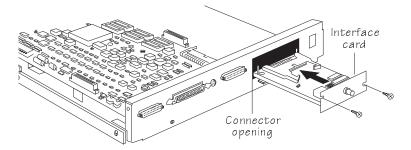
6 Using the two screws from the I/O plate you removed in step 2, mount the metal plate on the interface card to the connector opening.
