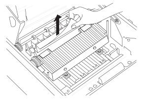
3 If the jammed media has passed completely through the fuser assembly and is partially visible in the upper output
