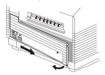
8 Remove the four screws holding the inner cabinet in place, and pull out the inner cabinet.
