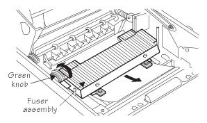
3 If the media is stuck in the rear of the fuser assembly, open the green fuser assembly rear door.
