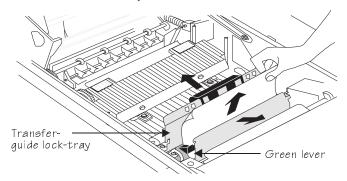
4 Restore the inner metal plate to its original position and close the transfer-guide lock-tray.
