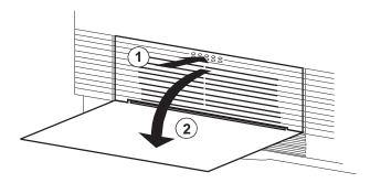
3 Carefully remove any jammed media. Then close the duplex access door.
