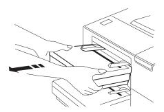
2 Remove the envelope feeder slot-cover located above the upper paper cassette slot by pushing it in and then down.
