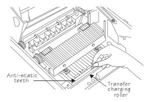
**Caution:** Be careful not to touch the transfer charging roller when cleaning the anti-static teeth. Finger oil, scratches, or other contaminants on the roller may reduce print quality.
