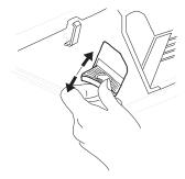
5 Pull the tab straight out. Pull the attached 22 inches (55 cm) of tape completely out of the cartridge. Discard the tab and tape.
