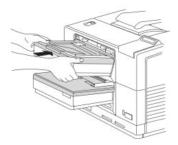
5 Take the envelope feeder in both hands, line up the positioning arms with the openings in the printer and insert the envelope feeder as far as it goes.
