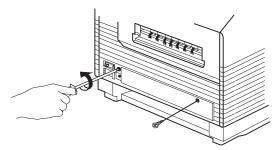
7 Push in a little on the right edge of the duplexing unit slotcover to unlock it. Then, slide the cover off to the right.
