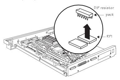
With the notched end of the new 220-ohm DIP resistor pack away from you (see the following illustration for orientation), carefully insert the resistor pack's pins in the RP1 socket where you just removed the 1 K-ohm resistor pack; then install the new 330-ohm DIP resistor pack in the RP2 socket, located next to the RP1 socket.
