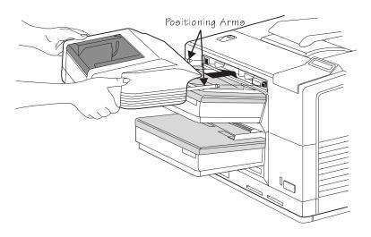
6 Open the envelope feeder cover and the envelope extension tray as shown.
