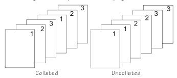
The face-down output bin has an offset stacking feature that when enabled, offsets the multiple copies of a print job. With a hard disk installed, collation performance is greatly improved because the file is stored in QMS-compressed format for repeated printing. When disk space is consumed during a print job, the printer begins chunk collating. Chunk collation breaks a job into sections and performs collation on each of those sections. The next diagram shows the printing
