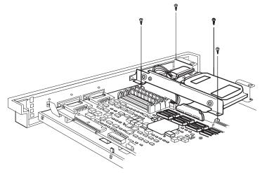
3 Disconnect the ribbon cable and power cable from the connectors on the controller board.
