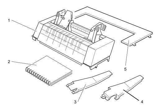
2 Attach the front and rear stacker supports to the sheet feeder.
