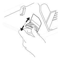
5 Firmly pull the tab and sealing tape straight out until all 22 inches (56 cm) of clear tape are completely out of the car-tridge.
