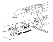
6 Make sure the toner cartridge is in position by pushing it in as far as it will go; then close the printer.
