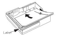
» Note: A label on the cassette shows which paper size to use. Use only that size. As a cassette is inserted in the printer, it sends an identifying signal to the printer's controller board so the printer can
