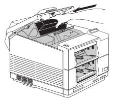
4 Grasp the tab protruding from the left side of the toner cartridge and flex it to break it loose.
