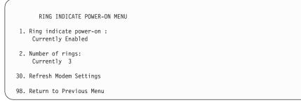
Ring indicate power-on is enabled by default on both serial port 1 (S1) and serial port 2 (S2). When ring indicate power-on is enabled, call-in is disabled.
