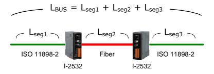
When users add one pair of I-2532 into a CAN bus system, the ideal bus length will reduce 50 meters because the propagation delay of one I-2532 is equal to the propagation delay caused by 25 meters bus length. For example, if users use baud 50Kbps and add two I-2532s into the CAN network, the ideal bus length should less than 950 meters (1000-25\*2=950).
