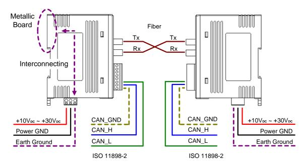
Roughly speaking, wiring of CAN\_GND and FG can improve the capability of anti-interference of CAN bus system, but this is not necessary.
