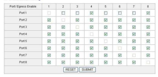
For example, in above figure, only the ingress come from Port 4 and Port 8 can be send out from Port 1.
