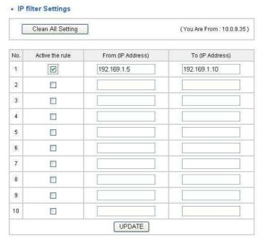
Before UPDATE the setting, you have to tick the <Active the rule> checkbox, otherwise system will ignore the setting data. You also can click the "Clean All Setting" button to reset the IP filter Table. Since the table is empty, system will allows all hosts to access the Switch.
