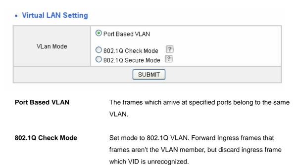
**802.1Q Secure Mode** Set mode to 802.1Q VLAN. Discard Ingress frames that frames
