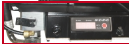
"SSPC" electronic pressure control and display
