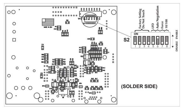
The table below shows the DIP Switch settings for McPC 10/100:
