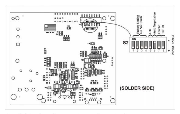
The table below shows the DIP Switch settings for McPC 10/100:
