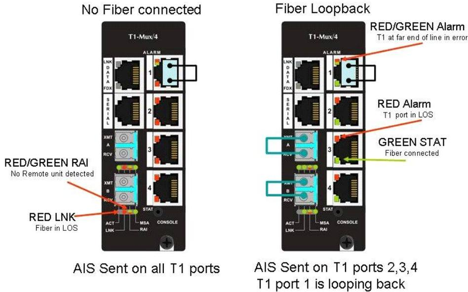
By placing a physical loopback connection on the T1 port, a valid signal can be detected by each individual T1 port to verify its operation. Without the fiber looped, the ALARM LED for the looped T1 port will show RED/GREEN indicating there is a problem at the far end of the fiber transport (In this case the far end unit is missing) and the STAT LED is RED because the fiber is in LOS. With the fiber looped, the T1 port will only show a normal GREEN STAT LED.
