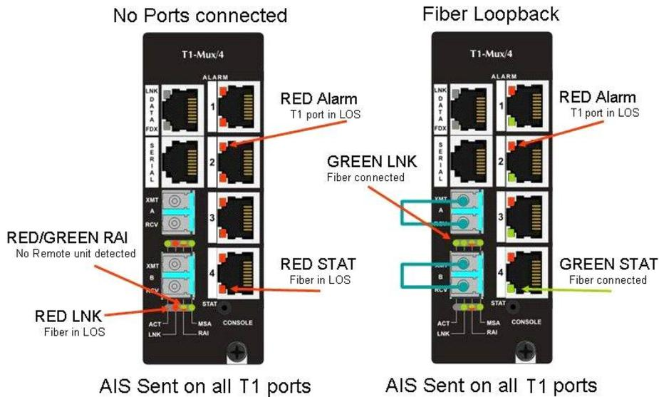
The *ACT LED* will arbitrarily be configured to either the A or B fiber line. The *RAI LED* is RED/GREEN indicating that there is something wrong at the far end of the fiber line (in this case, the remote unit is missing). The *ALARM LED* is RED because the T1 port is not connected. The *STAT LED* is RED when there is no fiber link but turns GREEN when the fiber link is valid.
