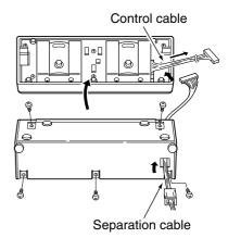
(7) Remove 2 screws from the cable hole cover on the linear amplifier rear panel. Insert the separation cable into the cable hole. Keep the hole cover and screws for future use.
