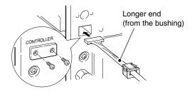
8 Plug the other longer end (from the bushing) of the separation cable into J10 on the JACK unit through the cable hole. Connect the grounding wire as shown below. Connect the control cable to J11.
