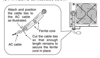
**NOTE:** Only one ferrite core is attached with the IC-PW1EURO.
