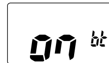
Battery voltage indication ON
