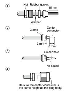
Slide the nut, flat washer, rubber gasket and clamp over the coaxial cable, then cut the end of the cable evenly.
