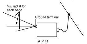
$^{1/4}\lambda$  (quarter wavelength) radial for each band is suitable for a counterpoise. Install the counterpoise directly below the AT-141's ground terminal. Insulate the ends of each radial from other metal objects. Layout the radial horizontally and as straight as possible.
